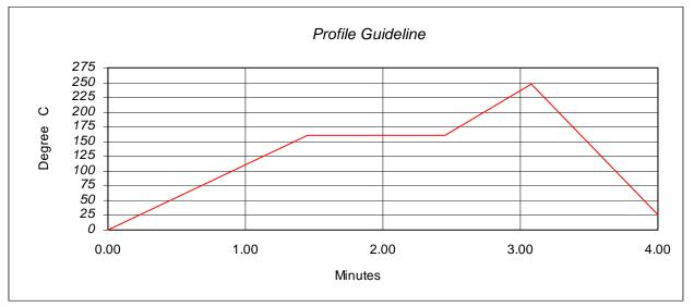
THE RECOMMENDED REFLOW PROFILE FOR NC257 IS PROVIDED AS A GUIDELINE. OPTIMAL PROFILE MAY DIFFER DUE TO OVEN TYPE, ASSEMBLY LAYOUT, OR OTHER PROCESS VARIABLES. CONTACT AIM TECHNICAL SUPPORT IF YOU REQUIRE ADDITIONAL PROFILING ASSISTANCE.
